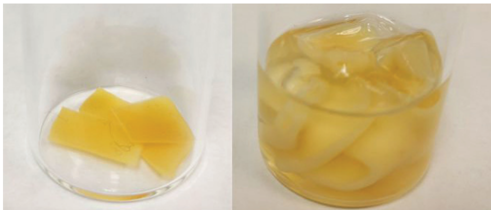
Figure 2. Dry soy-based SAP sample (left) and the same polymer sample swollen in water (right).
