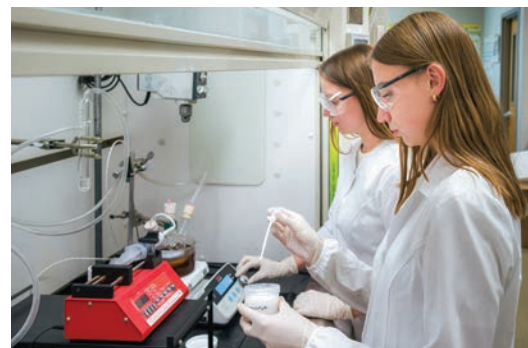
Figure 1. Coatings and Polymeric Materials graduate student Mariia Usiichuk (left) and summer student Yuliia Romaniuk synthesize highly soy-based latex PSAs.
