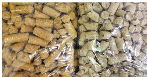
Figure 1. A visual comparison of the soybean meal and soyhull cube contrasted with the DDGS cube: the DDGS cube is slightly longer. The DDGS pellet did not hold up as well as the soy cube during the PDI test.
