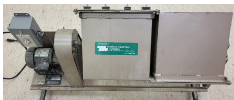
Figure 2. The tumble box was run for 10 minutes, with a 500-gram sample of each formula, to determine the pellet durability index.
