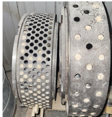
Figure 3. Surface area and pellet diameter comparisons of the two dies used.
