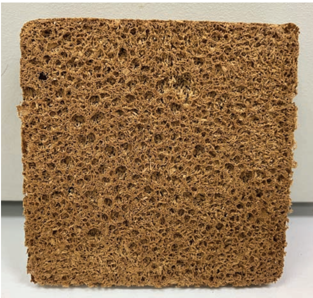
Figure 2. Cross section of foamed wood particle board that was made using this project's adhesive.
