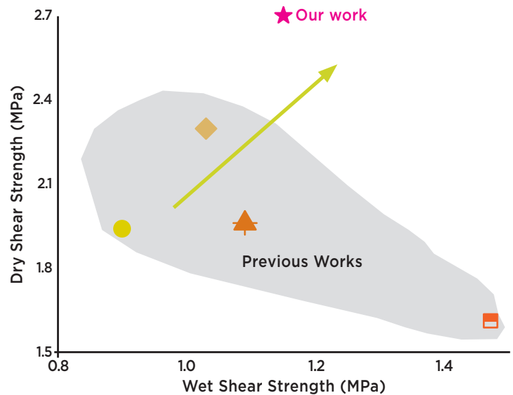
Figure 1. Comparison of dry and wet shear strength for the adhesives in this project and other studies.
