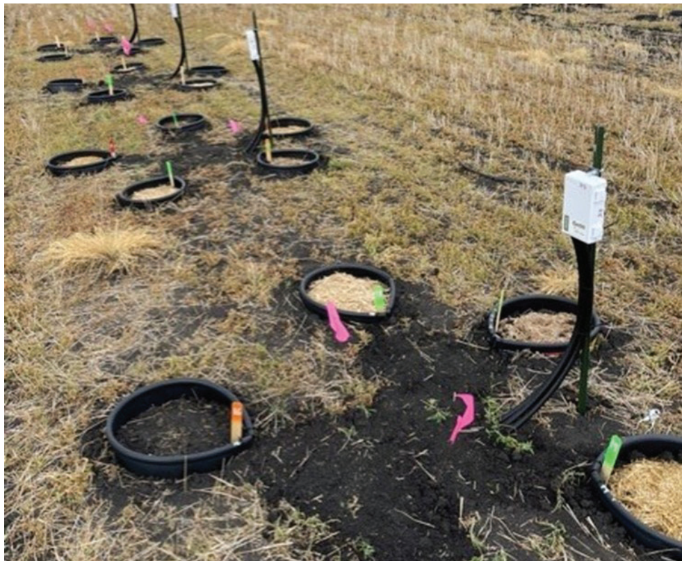
Figure 1. A microplot arrangement on a Fargo silty clay soil on the NDSU campus evaluated the seasonal soil moisture and temperature conditions that influence the soil's microbial activity and the rate of residue breakdown.
