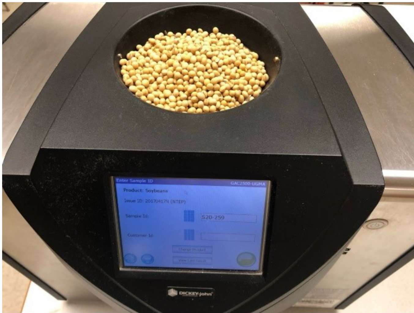
Image 1. Analysis of moisture and test weight of soybeans using a DICKEY-John Grain Analysis Computer
