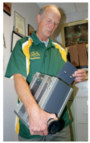
NDSU researcher Dr. Hans Kandel holds a tabletop control box. When connected to subsurface tile drainage, control boxes can help farmers manage the water table in their fields.
